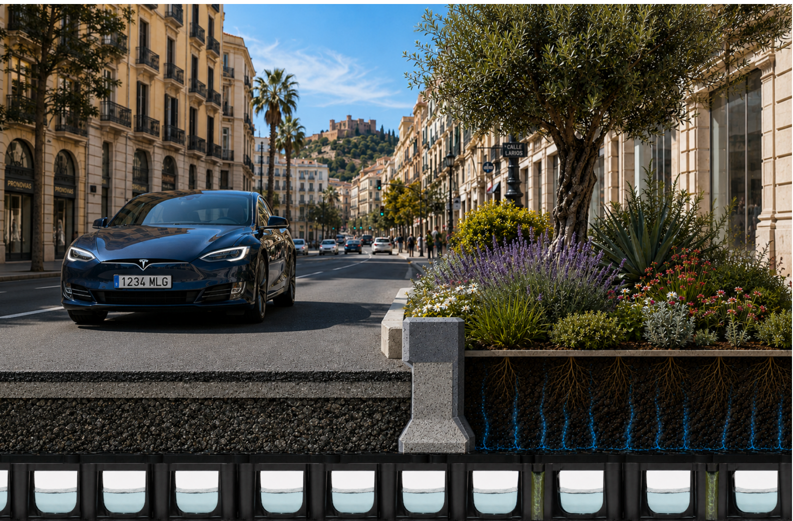
Figure 6. Lightweight water managing foundation combined with planters
